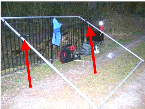
Picture 2: Trapping frame secured with mist net attached within (net still collapsed – see red arrows) immediately prior to net being extended.
