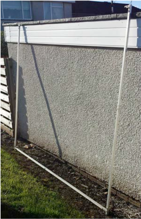
Picture 1: Aluminium frame extended in U configuration immediately prior to a mist net being placed within.
