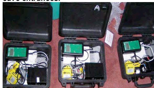
Figure 2 – Bat loggers within protective cases used at each of the cave entrances.
